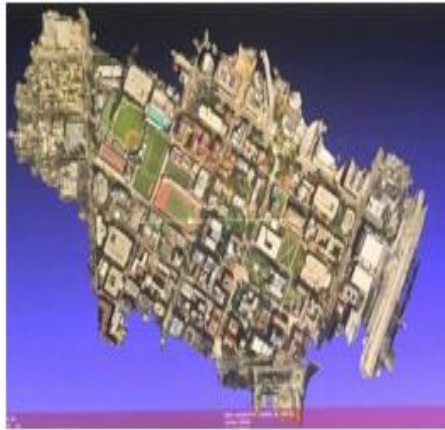
3D Model Reconstruction using Bundler & PMVS2
